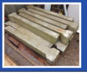
Single Rib Hammer-Head Slats • up to 10'6" (3195mm) length • 150mm thick • Ribs 130mm wide • Head 210mm wide to form 40mm gaps
